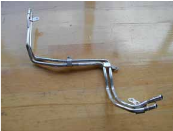
Picture 3 - Finished fuel lines
