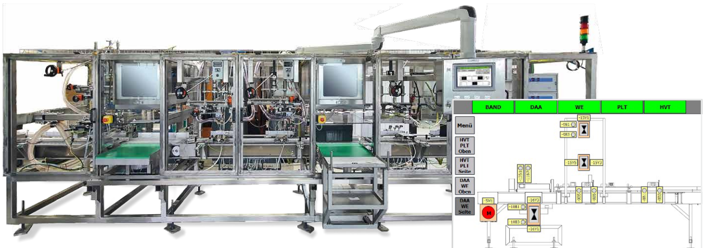
All machine components can be operated interactively, directly in an assembly drawing of the machine.
